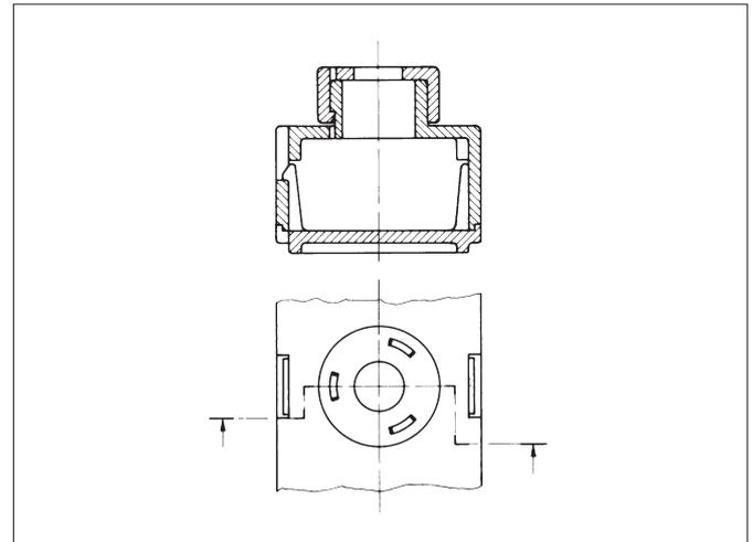
Fig. 9.22 **Micro-switch housing**
