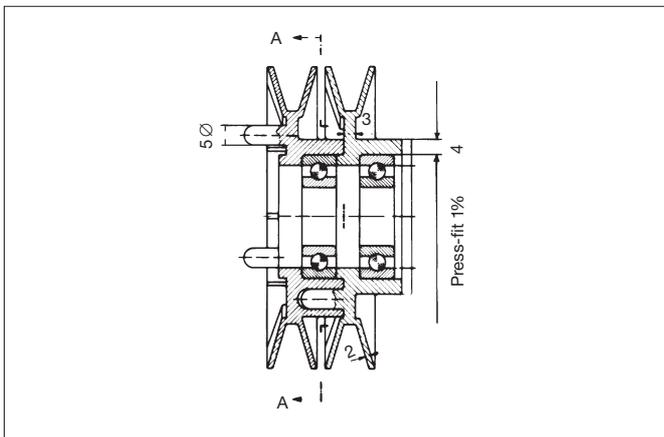
Fig. 9.15 Ball bearing
