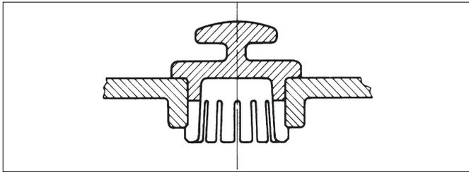
Fig. 9.26 **Slotted snap-fit**
