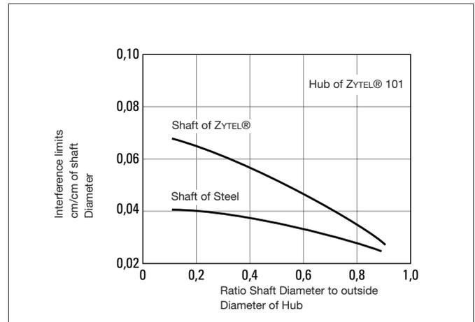
Fig. 9.10 Theoretical interference limits for press fitting
