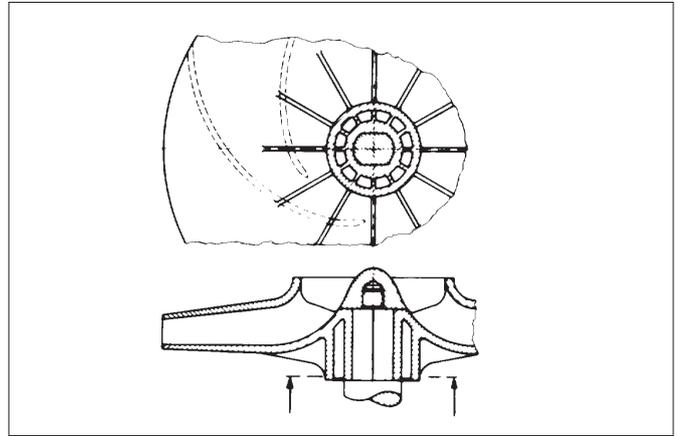
Fig. 9.34 **Outward-flow turbine**
