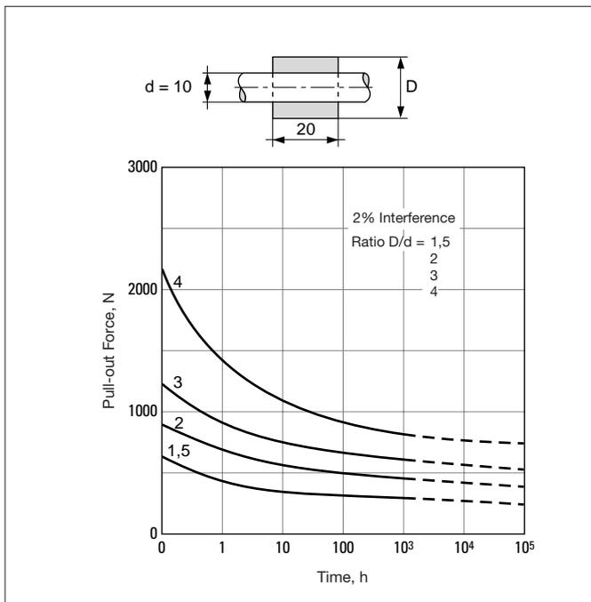
Fig. 9.11 Time vs joint strength – 2% interference
