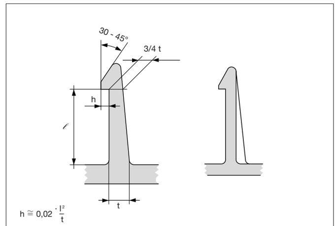
Fig. 9.17 Snap-fit cantilevered lug
