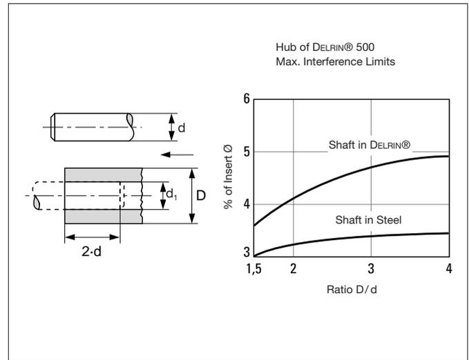
Fig. 9.09 Maximum interference limits
