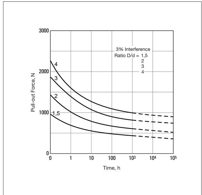
Fig. 9.12 Time versus joint strength – 3% interference
