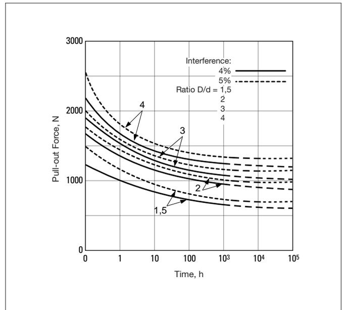
Fig. 9.13 Time versus joint strength – 4 and 5% interference
