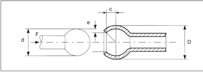
Fig. 9.18 Spherical snap-fit
