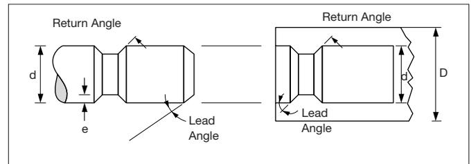
Fig. 9.16 Cylindrical snap-fit joint
