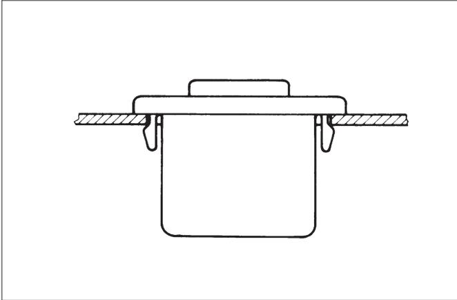
Fig. 9.24 Undersized snap-fit lugs
